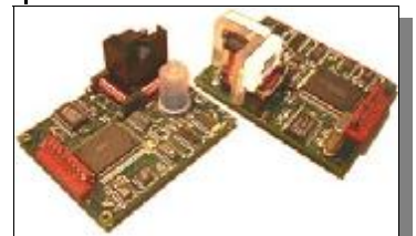
The TCM2 Electronic Compass, Magnetometer, and Tilt Sensor Module
