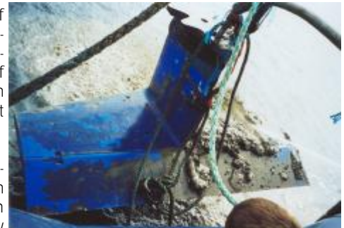
Recovered Hydrofoil. Note the Acoustic Locator Pinger attached on the middle of the elevator section.
