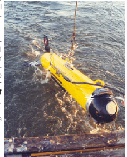
Deployment of The C3D Tow Vehicle During Sea Trial
