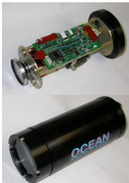
The DSC 4400 PCB board sets (above), and housing.
